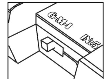
**Make sure put the G-M-I switch on the G mode before connecting to Android device. When connected, it can be switched between G mode and M mode. But if you pair it to Android device under I mode, it won't work when you switch the G-M-I switch to G mode directly. In this case, you must turn off the controller then put G-M-I switch to G mode to pair and connect Android device.**
